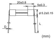
D L Rated current 100 mA-4 A:  $\phi$  0.5 30±5 Over 4 A-10 A:  $\phi$  0.8 40±5 Tube: Lead-free glass End-cap: Nickel plated brass Lead wire: Tin plated copper Sn-0.7Cu Solder: Adhesive: Epoxy resin (4) (§ SOC TSCR Marking:
