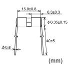
Tube: End-cap: Lead wire: Solder: Adhesive: Marking: Lead-free glass Nickel plated brass Tin plated copper 80 mA–1.25 A Over 1.25 A–5 A Epoxy resin SOC SU1 125V [rated current]
