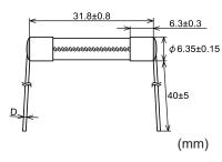
Rated current D 100 mA-8 A:  $\phi$  0.8 Over 8 A-15 A:  $\phi 1.0$ Over 15 A-30 A:  $\phi$  1.2 Tube: Lead-free glass Nickel plated brass End-cap: Lead wire: Tin plated copper
