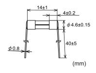
Tube: Lead-free glass End-cap: Nickel plated brass Lead wire: Tin plated copper
