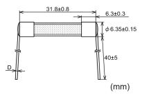
Rated current D 10 A:  $\phi$  1.0 Over 10 A-30 A:  $\phi$  1.2
