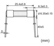
Tube:Lead-free glassEnd-cap:Nickel plated brassLead wire:Tin plated copperSolder:Pb90-Sn\*Adhesive:Epoxy resinArc extinguishing material:ConfidentialMarking:SOC [rated current]DC500V NSHV17
