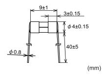
Tube: Lead-free glass End-cap: Nickel plated brass Lead wire: Tin plated copper Pb87.5-Sn10.0-Ag2.5\* Solder:
