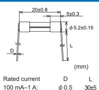
End-cap: Nickel plated brass Lead wire: Tin plated copper Solder: 100 mA–8 A Over 8 A–15 A Adhesive: Epoxy resin Marking: 100 mA–3.5 A Over 3.5 A–15 A
