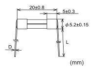
Rated current D L 62 mA-3 A:  $\phi$  0.5 30±5 Over 3 A-10 A:  $\phi$  0.8 40±5 Over 10 A-15 A:  $\phi$  1.0 40±5
