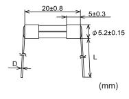
Rated current D L 62 mA-5 A:  $\phi$  0.5 30±5 Over 5 A-10 A:  $\phi$  0.8 40±5 Over 10 A-15 A:  $\phi$  1.0 40±5
