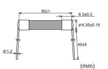
Tube:CeramicEnd-cap:Nickel plated brassLead wire:Tin plated copperSolder:3.15 A, 5 ASolder:20 A-35 AFAdhesive:Epoxy resinMarking:SOC [rated current]DC125V
