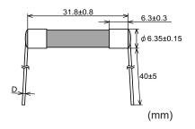
Rated current D 100 mA-8 A:  $\phi$  0.8 Over 8 A-30 A:  $\phi$  1.2 Tube: Ceramic
