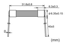
Rated current D 100 mA-8 A:  $\phi$  0.8 Over 8 A-25 A:  $\phi$  1.2 Tube: Ceramic
