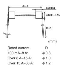
Tube: Lead-free glass End-cap: Nickel plated brass Lead wire: Tin plated copper Solder: 100 mA-12 A Sn-0.7Cu Over 12 A-30 A Pb90-Sn\*1 Adhesive: Epoxy resin Marking: 100 mA-less than 1 A SOC [rated current] 125V 1 A-30 A SOC [rated current] <₽>125V
