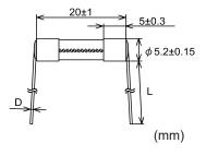
Rated current D L 100 mA-less than 5 A:  $\phi$  0.5 30±5 5 A-10 A:  $\phi$  0.8 40±5
