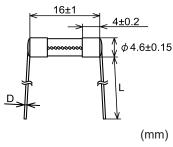
Rated current D L 100 mA-less than 5 A:  $\phi$  0.5 30±5 5 A:  $\phi$  0.8 40±5
