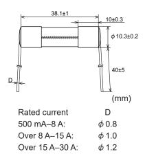
Tube: Lead-free glass End-cap: Nickel plated brass Lead wire: Tin plated copper Solder: 500 mA-12 A Sn-0.7Cu Over 12 A-30 A Pb90-Sn\*1 Adhesive: Epoxy resin Marking: 500 mA-less than 1 A SOC [rated current] 250V 250V 1 A-30 A SOC [rated current]
