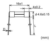
Rated current D L 100 mA-less than 5 A:  $\phi$  0.5 30±5 5 A:  $\phi$  0.8 40±5
