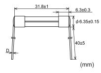
Rated current D 100 mA-8 A:  $\phi 0.8$ Over 8 A-15 A:  $\phi 1.0$ Over 15 A-20 A:  $\phi 1.2$  Tube: Lead-free glass
